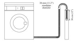
The standpipe should have an internal diameter of approximately 38mm (see diagram) thus ensuring there is an air break between the drain hose and standpipe.
